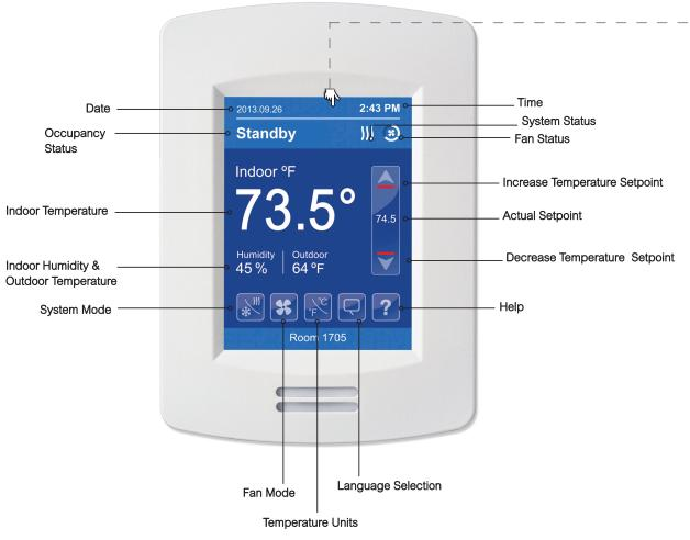
Touch and hold this point for 3 seconds to enter setup mode
