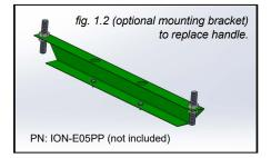
Remove the handle from the top of the unit by unfastening the two selftapping screws. Attach the mounting channel [figure 1.2] with the #8x1/2" self-tapping screws provided into the now vacant holes. Adjust the standalone air purifier to the desired height and secure in place by tightening two hex nuts along the allthread rods on both sides of the top flange.
