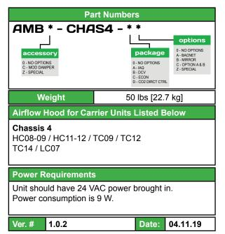
\*NOTE: Powered exhaust can be used with this hood.
